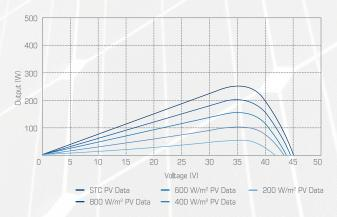
The typical change in the degree of module effectiveness with an irradiation of 200 W/m² instead of 1000 W/m² (both at 25°C and spectrum AM 1.5) < 3%
