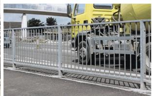
Designed to protect adults and children at road junctions and crossings, Pedestrian Guardrails are also ideal as perimeter fences to running tracks and play areas. Standard panels are 2m long and manufactured from 50 x 30mm RHS frame with either a 12mm or 16mm diameter infill set at 110mm centres. TRIAD can also manufacture Special Guardrail Panels to individual customer requirements ie raked and radiused panels.
